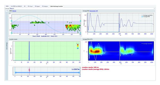
Manual parsing of the data is through the interactive graphical single line diagram. Any custom screens can be added to the software to represent the cable or substation components. A simple traffic light system shows the operator where to look for problems. The operator need only look at the more in depth data when needed, saving unnecessary time wasting.
